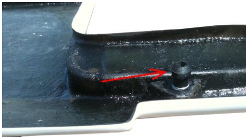
5. Installing cover by sliding back plastic tabs under black molding of car.
