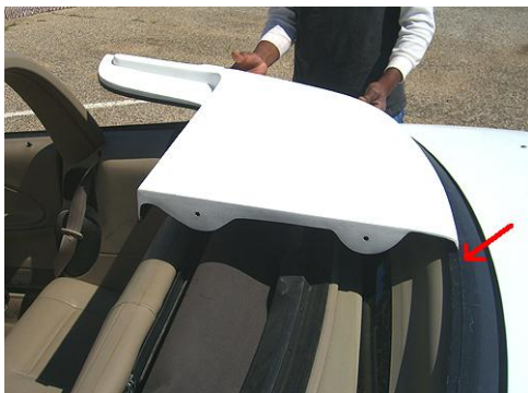
5. Installing cover by sliding back plastic tabs under black molding of car.
