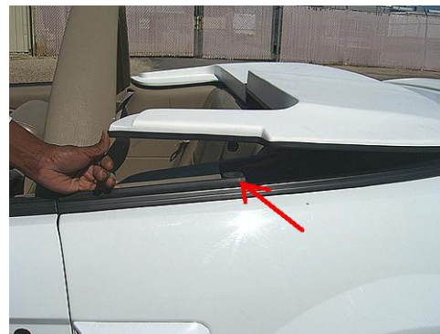
6. Installing front by pushing plastic ball studs into rubber sockets.
